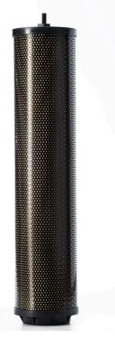
The Facet Flushing Filter elements are designed to be used in place of coalescer elements in a coalescer separator vessel during flushing on new systems or when there's been repairs to the existing equipment. The elements are less expensive than coalescer elements and have more filtration media for better solids holding capacity. Benefits, features and materials of construction are similar to our MP Series filter elements, except designed to flow inside to outside same as coalescer cartridges.
